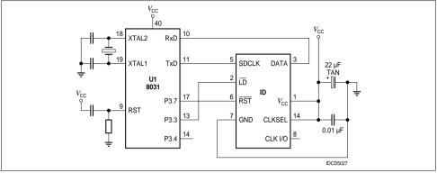
Display Interface to Siemens/Intel 8031 Microprocessor (using one bit of parallel port as serial port)
