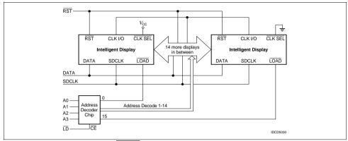
Multiple displays can be cascaded using the CLK SEL and CLK I/O pins (Figure "Cascading Multiple Displays using only the SCE574X" (page 13)). The display designated as the MasterClock source should have its CLK SEL pin tied high and the slaves should have their CLK SEL pins tied low. All CLK I/O pins should be tied together. One display CLK I/O can drive 15 slave CLK I/Os. Use RST to synchronize all display counters.
