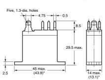
Mounting Holes (BOTTOM VIEW) Tolerance: ±0.1 mm
