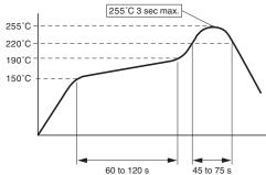
The peak temperature may vary depending on the reflow bath used. Confirm the conditions beforehand.
