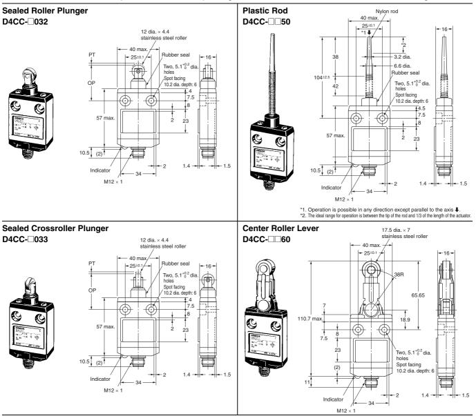
The in each model number is replaced with the code expressing the rated load of the model. Refer to Model Number Legend.
