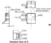
Note: 1. Use M3 or M2.6 pan screw or tapping screw with an equal diameter for installation. And bind tight with 0.59N·m or less torque.
