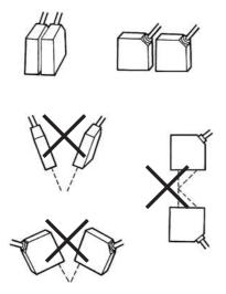
When using the LED Displacement Sensor in combination with another type of Sensor (such as a Photoelectric Sensor), the sensor beams should be as close to perpendicular as possible.
