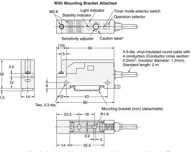
\*After adjusting the sensitivity, attach the caution label at the location indicated by  $\bigcirc$  above to prevent malfunction.
