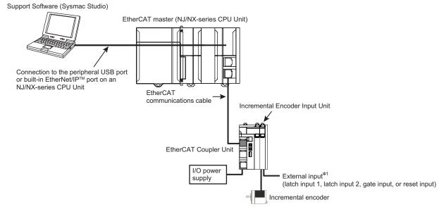
\*1. You can specify functions for up to two external inputs to a One-input Incremental Encoder Input Unit. You cannot use external inputs for a Two-input Unit.
