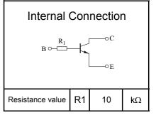
Transistors with Built-in Resistor
