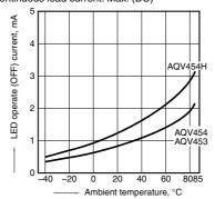
6. LED reverse (ON) current vs. ambient temperature characteristics Load voltage: Max. (DC);
