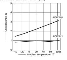
2.-(2) On resistance vs. ambient temperature characteristics
