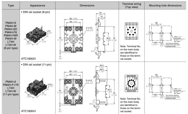
Note: The socket's numbering system matches that of the timer terminals.
