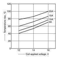
1.-(2) Coil temperature rise (85°C 185°F) Sample: CP1-12V, 6pcs Point measured: Inside the coil Contact carrying current, 5A, 10A, 15A, 20A Resistance method, ambient temperature 85°C 185°F
