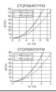
PWB condition A : Four-layer PWB (1.6 mm FR4), See also (\*2) PWB condition B : Multilayer PWB with high heat dissipation performance. See also (\*3)
