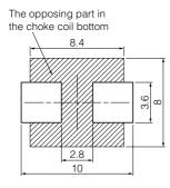
③ Parts arranged around this power choke coil do not touch the surface of this power choke coil (Top side and side). (Series MC)
