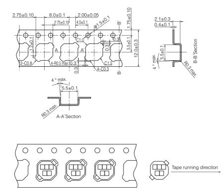
Embossed Carrier Tape Dimensions in mm (not to scale)
