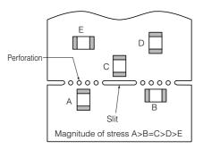
(3) The magnitude of mechanical stress applied to the Inductors when the circuit board is divided is in the order of push back < slit < V-groove < perforation.</p>
