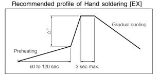
$\triangle T$  : Allowable temperature difference  $\triangle T \leq 150 \ ^{\circ}C$
