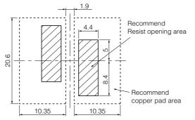
Due to bigger part, Thermal Capacity is large and may occure PWB temperature differences during reflow process. Recommended land pattern (Heat absorb) should be
