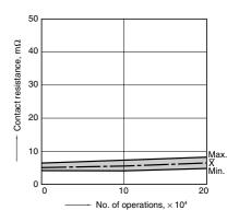
6-(2). Electrical life test (Motor lock) Sample: ACT212, 3pcs. Load: 25A 14V DC Power window motor actual load (lock condition)
