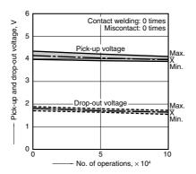
6-(2). Electrical life test (Lamp load) Sample: JSM1a-12V-5, 4pcs. Load: 55.2A (Inrush), 9.6A 14.5V DC (Steady) Switching frequency: (ON: OFF = 1s: 3s)
