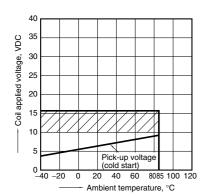
4. Distribution of pick-up and drop-out voltage Sample: JSM1-12V-5, 50pcs.
