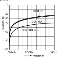
1-(2). High frequency characteristics (Impedance  $75\Omega$ )
