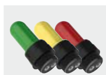
Light indicators A light indicator is used in order to visualize a change of state of the electric contacts inside the switch. It can be installed only in the series FL, FX, FZ or FS by screwing it on one of the conduit entries not used for electric cables. Protection degree IP67.
