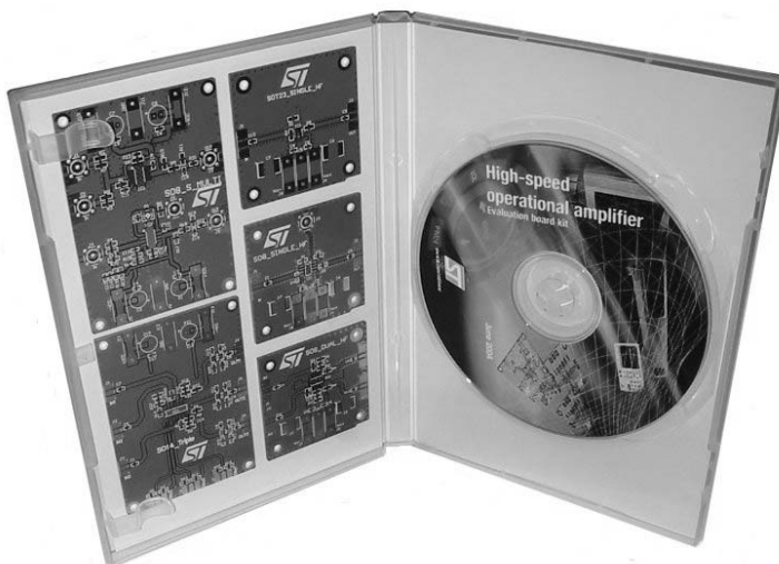
Figure 22: Evaluation kit for high speed op-amps
