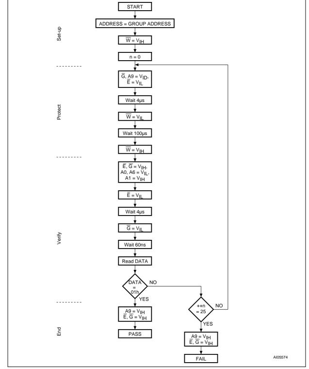
Figure 19. Programmer Equipment Group Protect flowchart
