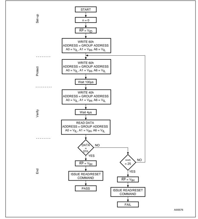
Figure 21. In-system Equipment Group Protect flowchart
