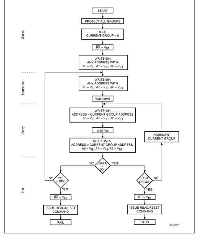
Figure 22. In-system Equipment Chip Unprotect flowchart
