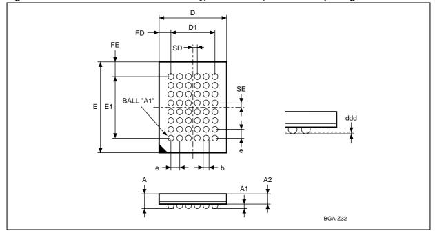
Figure 18. TFBGA48 6x8mm - 6x8 Ball Array, 0.8mm Pitch, bottom view package outline
