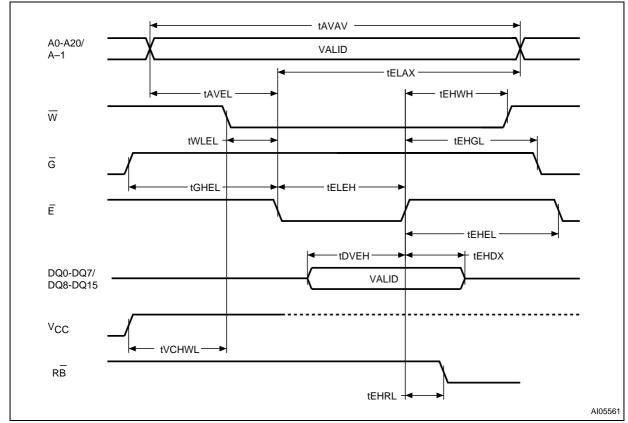
Figure 12. Write ac waveforms, Chip Enable controlled
