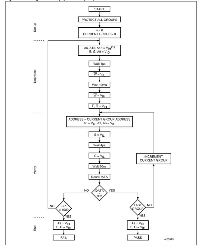
Figure 20. Programmer Equipment Chip Unprotect flowchart
