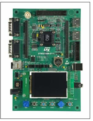
designed to help developers evaluate all device peripherals (such as HDMI CEC, motor control, LCD, microSD Card<sup>™</sup>, serial Flash, speaker, IrDA and USART) and develop their own applications.
