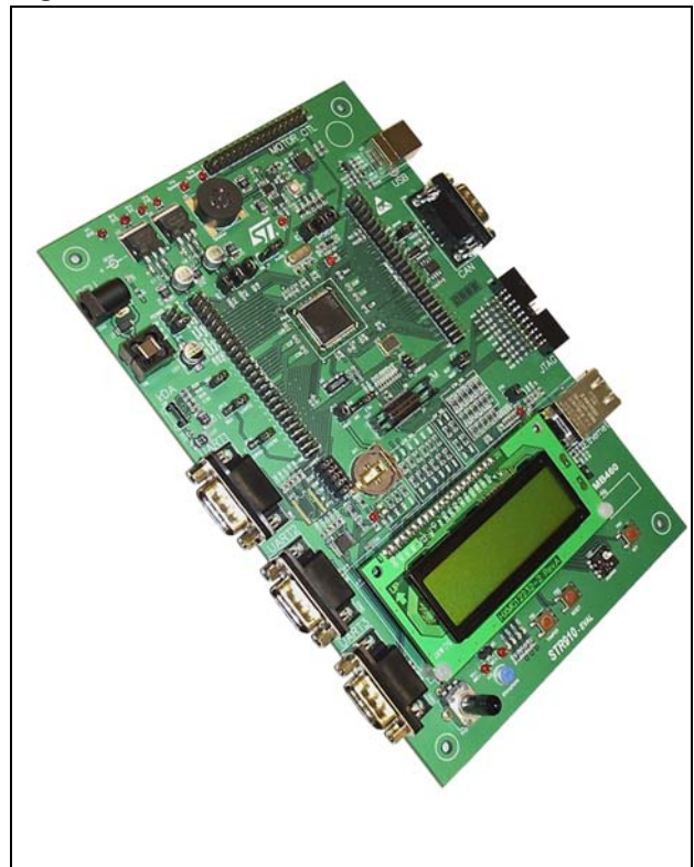
Figure 1. STR910 evaluation board
