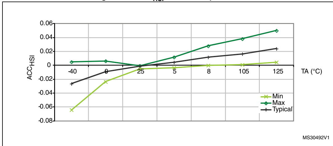
Figure 26. ACC HSI versus temperature
