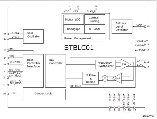
Figure 3. Simplified block diagram
