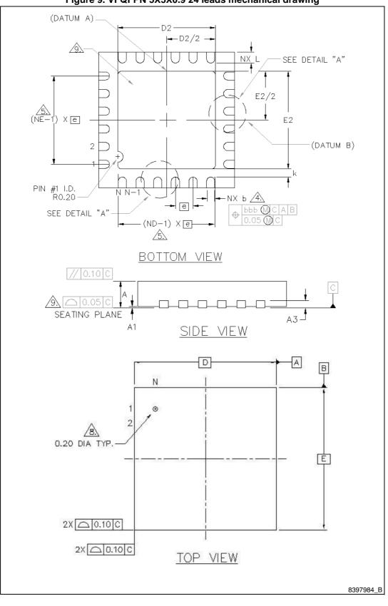
Figure 9. VFQFPN 5X5X0.9 24 leads mechanical drawing
