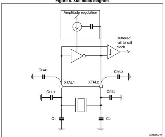
Figure 8. Xtal block diagram
