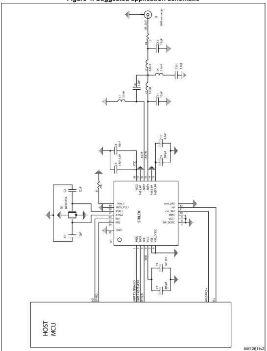
Figure 4. Suggested application schematic
