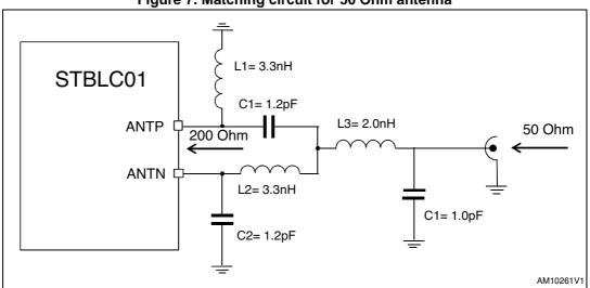
Figure 7. Matching circuit for 50 Ohm antenna
