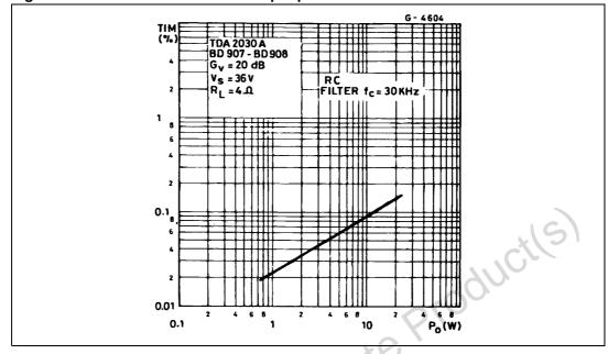
Figure 28. TIM distortion versus output power
