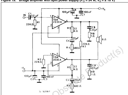
Figure 19. Bridge amplifier with split power supply ( $P_O = 34 \text{ W}$ ,  $V_S = \pm 16 \text{ V}$ )
