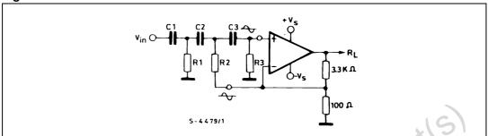
The proposed circuit can realize combined power amplifiers and 12 dB/octave or 18 dB/octave high-pass or low-pass filters.
