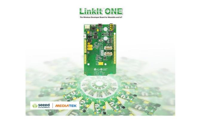
The LinkIt ONE development platform is an open source, high performance board for prototyping Wearables and IoT devices. It is based on the world's leading SoC for Wearables, MediaTek Aster (MT2502) combined with high performance Wi-Fi (MT5931) and GPS (MT3332) chipsets to provide you with access to all the features of MediaTek LinkIt. It also provides similar pin-out features to Arduino boards, making it easy to connect various sensors, peripherals, and Arduino shields.
