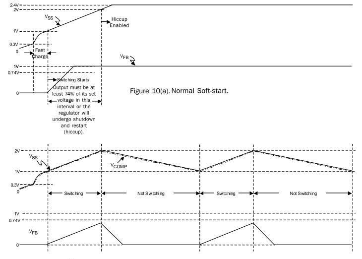
Figure 10(b). Start-up Fails due to (i) Short Soft-start Duration or (ii) Output Overload or (iii) Output Short-circuited.
