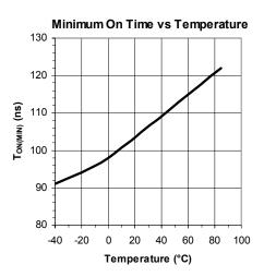
Figure 6. Variation of Minimum On Time with Temperature.
