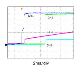
CH1: OUT1 Voltage, 0.5V/div CH2: OUT2 Voltage, 1V/div CH3: SS2 Voltage, 1V/div CH4: PGOOD2, 1V/div
