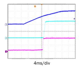
Upper Trace :  $V_{IN}$ , 10V/div Middle Trace :  $V_{OUT1}$ , 2V/div Lower Trace :  $V_{OUT2}$ , 1V/div
