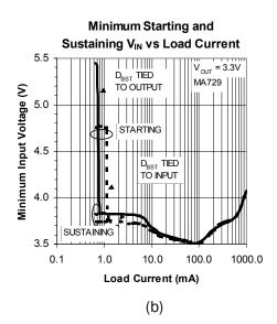
Figure 9. Minimum Input Voltage Required to Start and to Maintain Bootstrap.( $T_A = 25$ °C).
