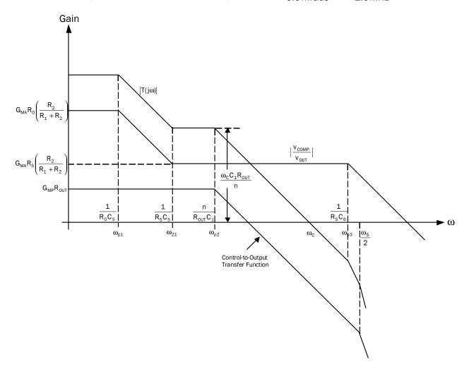
Figure 13. Bode Plots of Control-to-Ouput, Output-to-Control and the Overall Loop Gain. Control-to-output transfer function is shown with two poles near half the switching frequency  $\omega_{\rm e}$ .
