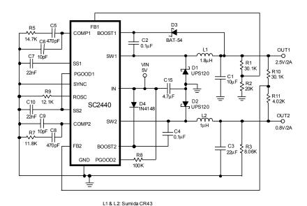
Figure 18(a). Producing an Output Lower than FB Voltage. 1.5MHz 5V to 2.5V and 0.8V Step-down Converter  $R_3$  is a pre-load to shunt the current from  $R_{10}$  and  $R_{11}$  before PGOOD1 releases SS2.
