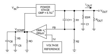
Figure 12. Simplified Control Loop Equivalent Circuit
