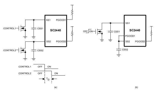
Figure 11. Sequencing the Outputs by (a) Delaying Release of one Channel Relative to the Other and (b) Using the PGOOD of one Channel to Control the Other.
