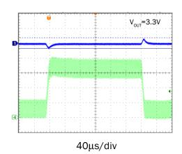
Upper Trace : OUT1 Voltage, AC Coupled, 0.5V/div Lower Trace : L₁ Inductor Current, 0.5A/div
