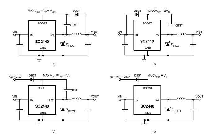
Figure 8. Methods of Bootstrapping the SC2440.
