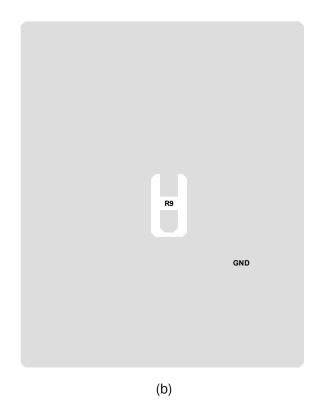
Figure 16. Suggested PCB Layout for the SC2440. Notice that there is no via directly under the device and that the only component on the backside is the frequency-setting resistor. All vias are 12mil in diameter.
