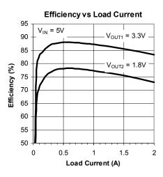
Figure 17(a). 1.3MHz 5V to 3.3V and 1.8V Step-down Converter
