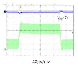
Upper Trace : OUT2 Voltage, AC Coupled, 0.5V/div Lower Trace : L<sub>2</sub> Inductor Current, 0.5A/div
