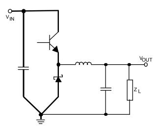
Figure 15. Fast Switching Current Paths in a Buck Regulator. Minimize the size of this loop to reduce parasitic trace inductance.
