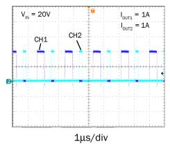
CH1: SW1 Voltage, 10V/div CH2: SW2 Voltage, 10V/div
