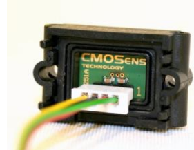
Figure 2 Pin assignment of SDP6xx on PCB top view from left to right. Connect cable such that yellow cable is connected to data, black (GND), red (Vdd) and green (clock).
