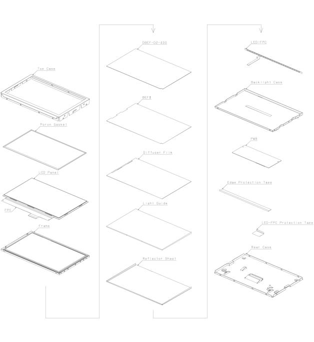
Fig. 4 Construction of LQ080Y5DZ03
