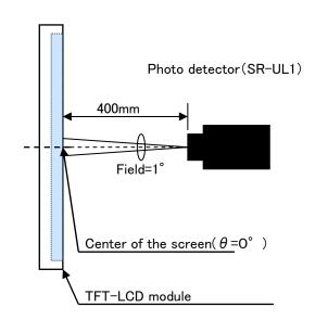
Fig. 7 The way of measuring Luminance/ Chromaticity/ Contrast
