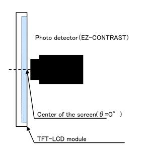
Fig. 6 The way of measuring
