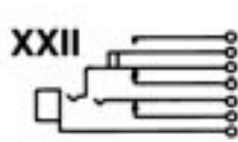
Double closed circuit. Isolated switching "make" circuit on ring spring. (J7-1A).
