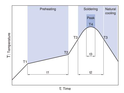
Preheating Soldering Peak Temp. Temp. Time Time Temp. Time T1 T2 T4 Т3 t3 150°C 180°C 60 to 120s 230°C 30s 260°C 10s
