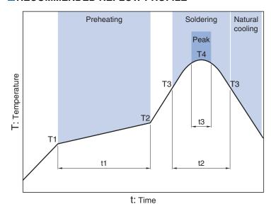
Preheating Soldering Peak Time Temp. Time Temp. Temp. Time T1 T2 T4 T3 t3 150°C 180°C 90 to 120s 230°C 40s 255°C 10s max.
