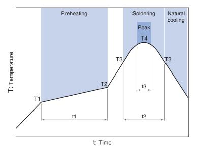
Preheating Soldering Peak Temp. Temp. Time Temp. Time Time T1 **T2** t1 Т3 t2 **T**4 t3 150°C 180°C 60 to 120s 230°C 10 to 30s 245°C 5s max. (4/11)
