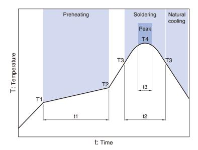
Preheating Soldering Peak Temp. Temp. Time Time Temp. Time T1 T2 **T4** Т3 t3 130°C 150°C 110s 200°C 260°C 90s 5s
