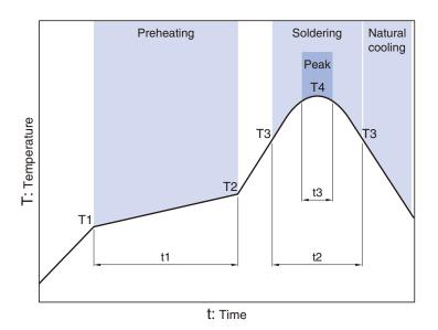
Soldering Preheating Peak Temp. Temp. Time Time Temp. Time T1 **T2 T**4 t1 ТЗ t2 t3 150°C 180°C 60 to 120s 230°C 260°C 30s 10s
