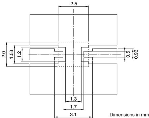
Line width be designed to match 50Ω characteristic impedance, depending on PCB material and thickness.
