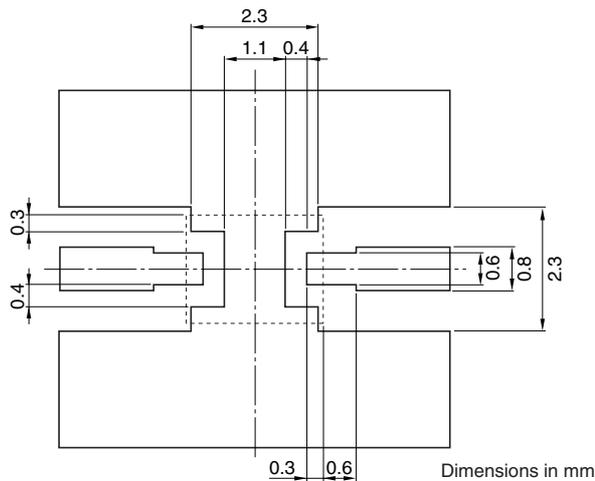
Line width be designed to match 50Ω characteristic impedance depending on PCB material and thickness.
