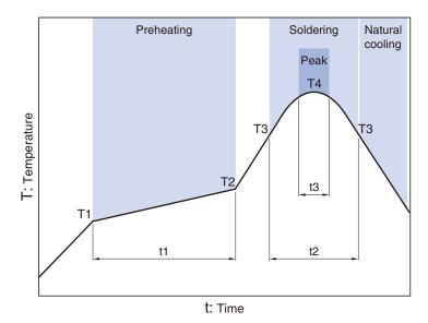
Soldering Preheating Peak Temp. Temp. Temp. Time Time Time T1 T2 T4 t3 Т3 150°C 180°C 60 to 120s 230°C 250 to 260°C 30 to 60s 10s max.
