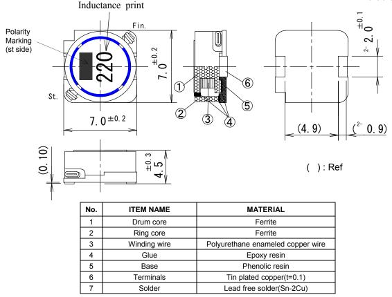
Note: 1) It is acceptable even if adhesive is out of ring core, but it shouldn't be out of base. Note: 2) Even if the adhesives of an upper surface application have the portion which has not been buried completely, they presuppose that it is possible.
