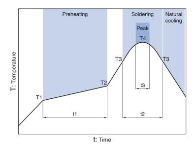
Soldering Preheating Peak Temp. Temp. Temp. Time Time Time T1 T2 Т3 **T**4 t3 150°C 180°C 60 to 120s 230°C 30 to 60s 250 to 260°C 10s max.
