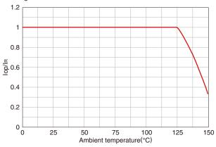
$\bigcirc$  Maximum current value for the ambient temperature (mA)
