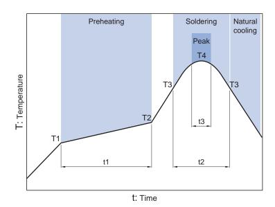
Preheating Soldering Peak Temp. Temp. Time Time Temp. Time T1 T2 T4 Т3 t3 150°C 180°C 120s 230°C 260°C 10s max. 30s
