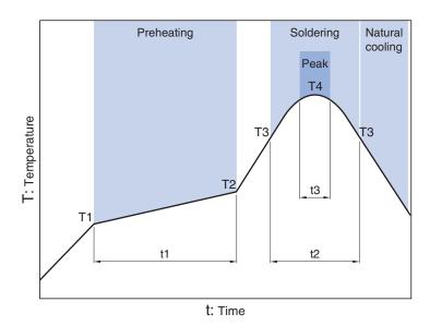
Preheating Soldering Peak Temp. Temp. Time Temp. Time Time T2 T3 T4 t3 180°C 150°C 90 to 120s 40s 230°C 255°C 10s max.
