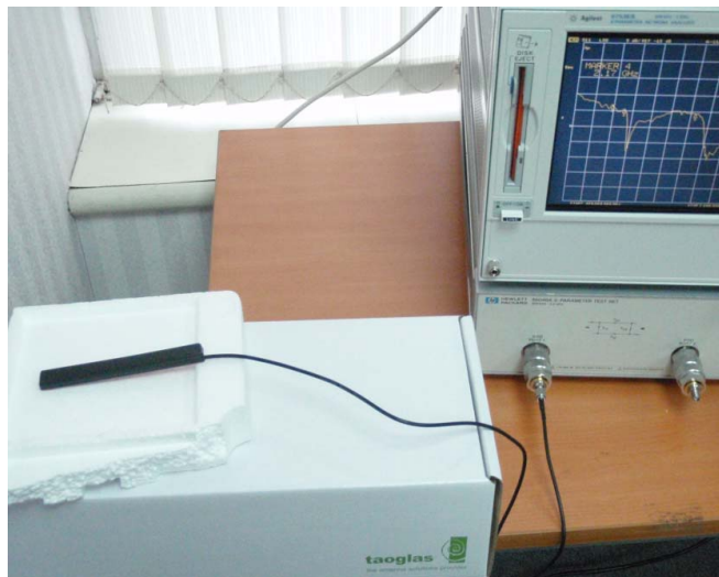
Free space Return Loss measurement setup
