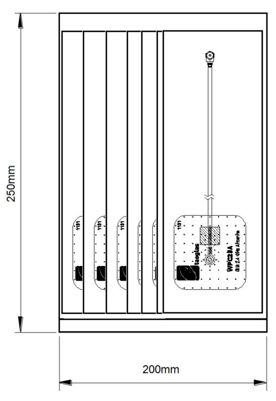
10 Antennas are then packaged in an Outer PE Bag: 250mm\*200mm
