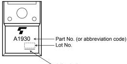
A line indicates lead (Pb)-free package or lead (Pb)-free finish.
