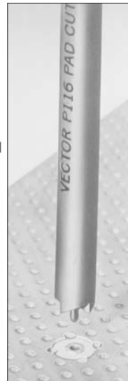
Shows pad removal & pad cutter P116C
