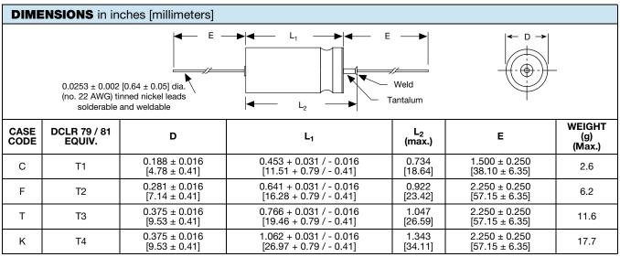
• For insulated parts, add 0.015" [0.38] to the diameter. The insulation shall lap over the ends of the capacitor body.
