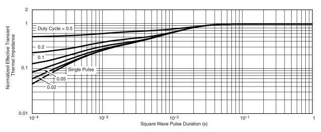
Normalized Thermal Transient Impedance, Junction-to-Case
