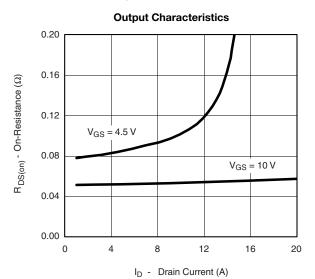
On-Resistance vs. Drain Current
