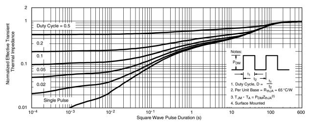
Normalized Thermal Transient Impedance, Junction-to-Ambient
