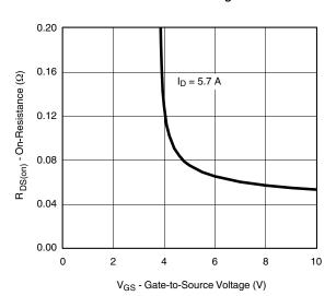
On-Resistance vs. Gate-to-Source Voltage
