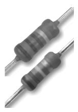
A homogenous film of metal alloy is deposited on a high grade ceramic body. After a helical groove has been cut in the resistive layer, tinned electrolytic copper wires are welded to the end-caps. The resistors are coated with a blue, non-flammable lacquer, which provides electrical, mechanical, and climatic protection.
