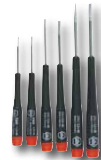
26090 6 Piece Precision Slotted Set Blade high alloy chrome-vanadium-molybdenum steel. Hard chrome finished. Item No. Blade Size Weight (lbs.) 26090 Slotted: 1.5, 2.0 x 40mm .27 2.5, 3.0 x 50mm 3.5, 4.0 x 60mm
